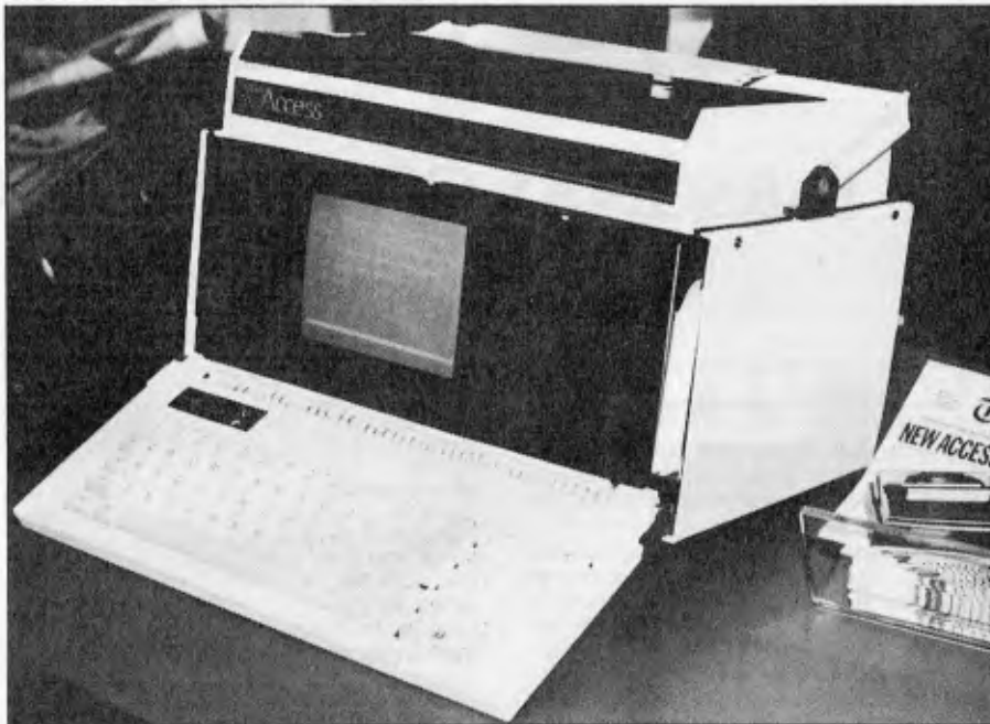
One of the host of new portables around was this one, the Access, which comes complete with a dot matrix printer welded onto its top, making it even less portable (because of its weight and power requirements) than most.
